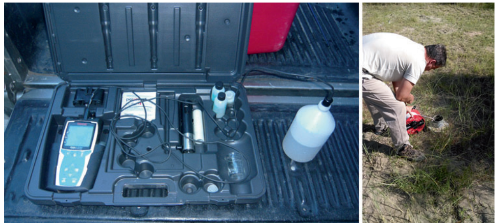
Borehole Investigations, Fig. 2 Water samples and water table measurement
