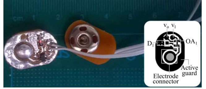
Fig. 6. Photograph of the implemented active electrode with two-wire leads. The inset shows the PCB layout and component placement.
