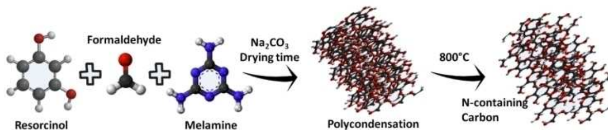
Figure 1. Scheme of the one-step synthesis reaction.
