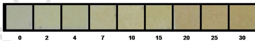
Fig. 2. Photograph of PU films after different exposition times (minutes) under UV light.
