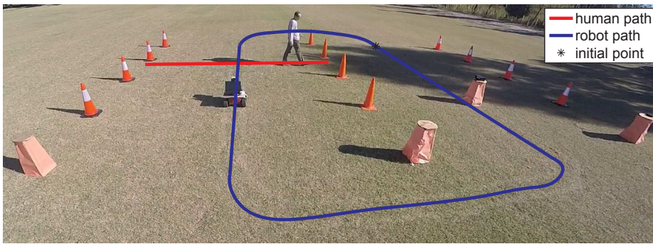
Fig. 9. Experimental environment constructed using red traffic cones and stools as fruit trees and static obstacles. The robot must cyclically follow a path (blue line), evading a static obstacle in the first row, and a dynamic obstacle (worker going back and forth along the red line) in the second row. (For interpretation of the references to color in this figure legend, the reader is referred to the web version of this article.)
