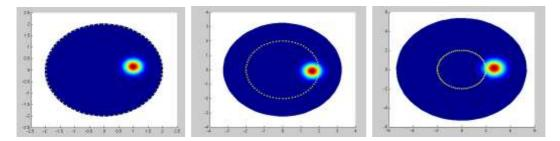
Fig. 7.7 Solution using Moving Mesh with and explicit integration of the particle position after 1,2 and 3 flow tours. (LMM-1)
