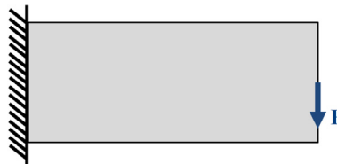
Fig. 7. Schematic drawing of a cantilever beam with homogeneous material distribution.
