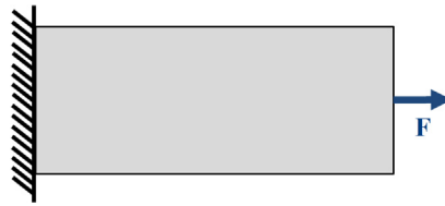
Fig. 5. Schematic drawing of a traction rod with homogeneous material distribution.
