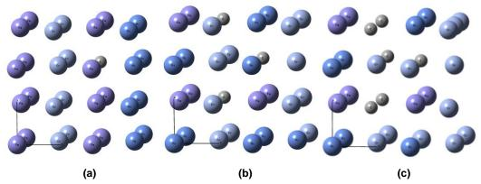
Figure 6. Schematic view of (a) HP, (b) M7C3 and (c) M23C6 models.
