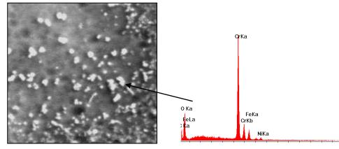
Figure 5. Secondary precipitation of carbides in an over-aged sample.
