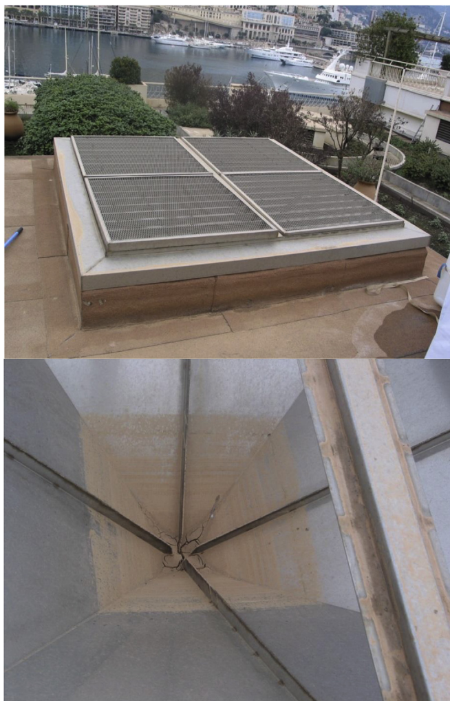
Fig. 2. Stainless steel collector on the roof of IAEA-EL premises in Monaco for collection of dry and wet deposits (Note in the lower part shown the important residue of dust deposition SD1 collected on the 20 February 2004).
