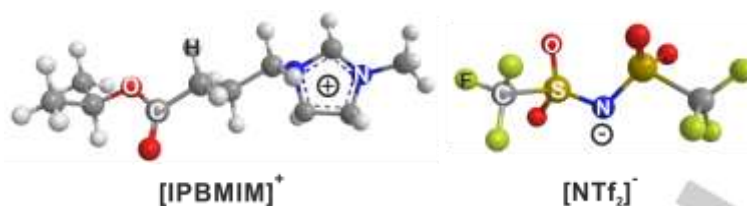
Scheme 1 Molecular structure of 3-(4-isopropoxy-4-oxobutyl)-1-methylimidazolium bis(trifluoromethylsulfonyl)imide ([IPBMIM][NTf 2 ]).
