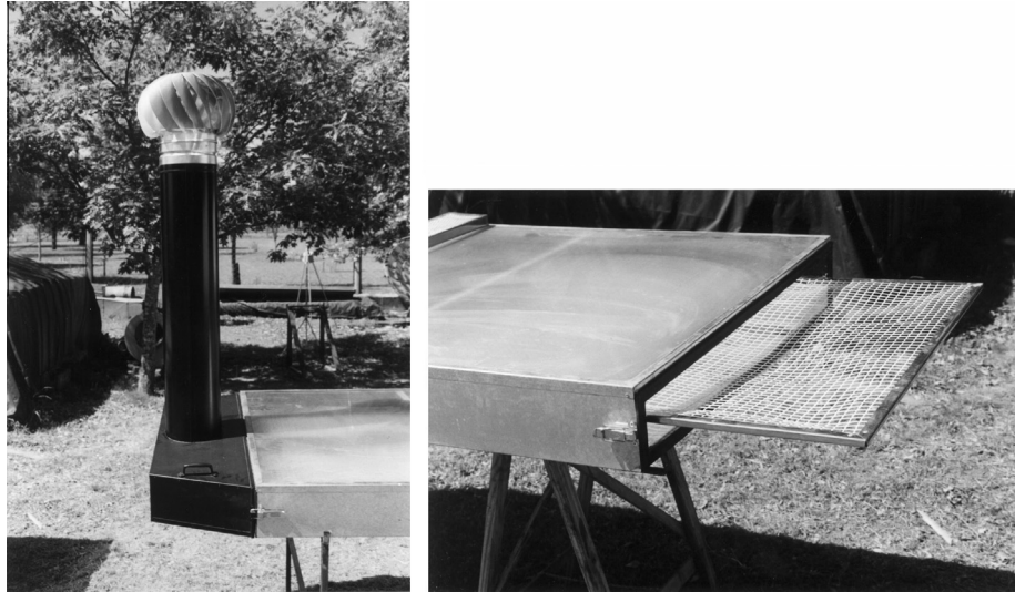
Fig. 1. Photo of passive solar dryer. Back of chamber with elbow union, chimney and wind turbine (left); front part of chamber with plastic tray (right).
