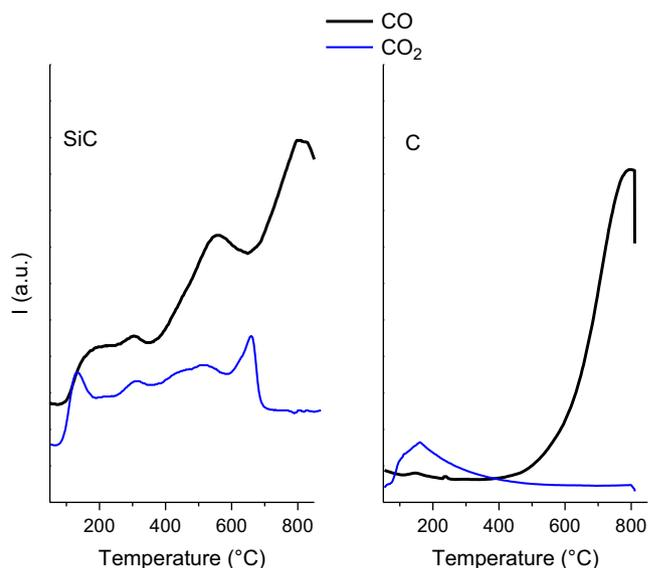
Fig. 2. Temperature programmed desorption (TPD). TPD spectra (in helium flow) of SiO<sub>2</sub>-C and C supports: CO (—) and CO<sub>2</sub> (—) released.
