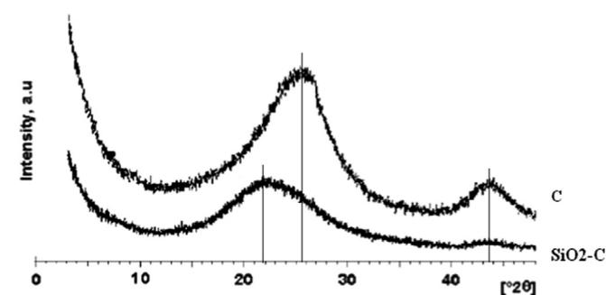
Fig. 1. XRD patterns for SiO<sub>2</sub>-C and C materials.
