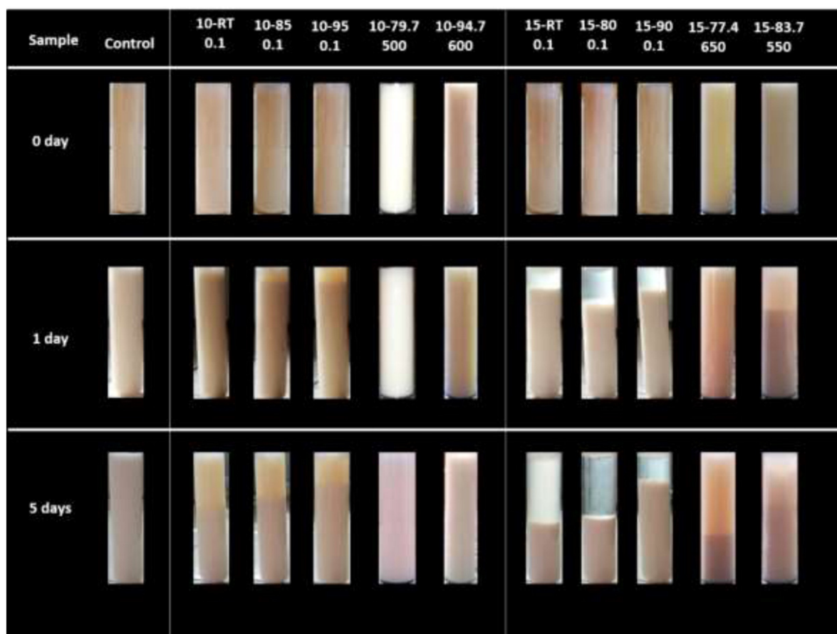
Fig. 4. Phase separation in soymilks subjected to different treatments after 0, 1 and 5 days. RT: room temperature. Figures correspond to \text{CaCl}_2 concentration ( \text{mmol L}^{-1} ), temperature (thermal treatment at 0.1 MPa or process temperature of HHP treatments, ^{\circ}\text{C} ) and pressure level (MPa), respectively.
