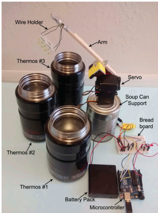
Figure 2. Thermos thermal cycler (TTC) setup with three thermos for amplification rounds that require three distinct temperatures. Components shown in the picture include three thermoses, a pan-and-tilt servo to motion the PCR tubes between them, the Arduino electronic controller, a breadboard, and a battery pack. In order to reduce costs, the pan-and-tilt setup is constructed using a soup can and a wood stick, and the PCR tubes holder is made with metal wire. Figure reproduced from reference [71] under the terms of the Creative Commons Attribution License © 2016 Chan et al.
