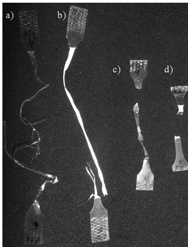
FIG. 3. Tensile samples: (a) PP, (b) PP-5 longitudinal direction, (c) PP, and (d) PP-5 transversal direction.
