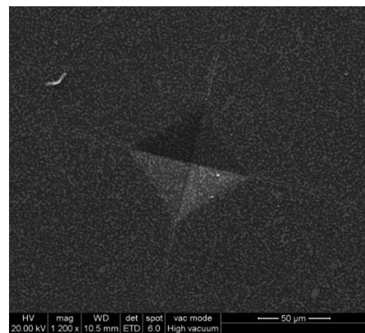
Fig. 6. SEM image of the Vickers indentation of the mullite–zirconia material sintered at 1500 °C with a 10 min soaking.
