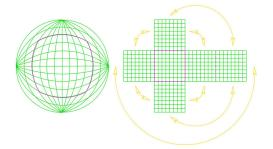
FIG. 1 (color online). Cubed sphere coordinates. A total of six Cartesian patches are employed to cover the sphere. Only patch boundaries coincide at common points.
