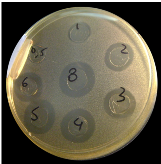
Fig. 2. Inhibition areas exerted by multilayer-LLDPE film treated with 0.5; 1; 2; 3; 4; 5; 6; 8 µg ml -1 of S-705.
