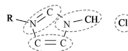
Fig. 4. Groups contained within the [-mim][Cl] group for evaluating parameters r_{[-mim][Cl]} and q_{[-mim][Cl]} .
