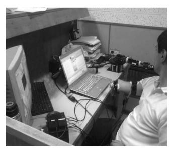
**Fig. 13.** The user had to control the robot through muscle contraction and visual feedback to confirm the correct movements. The task involved a sequence of pronation, supination, flexion, extension movements interspersing with short rest intervals.
