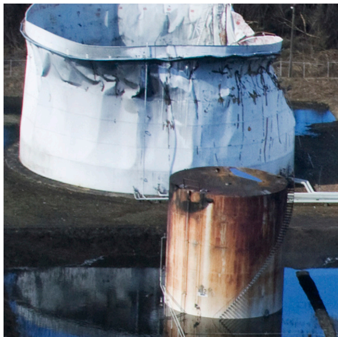
Fig. 5. Deformed configuration of a tank without external fixed roof after the Bayamon accident occurred in 2009
