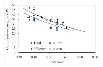
Figure 2. Relationship between compressive strength and total and effective w/c ratios.
