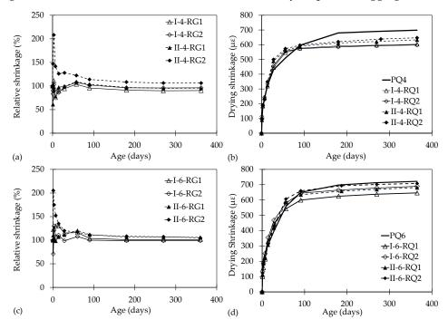
**Figure 5.** Drying shrinkage development over time. (a) Granite concretes, w/c = 0.40. (b) Quartzite concretes, w/c = 0.40. (c) Granite concretes, w/c = 0.55. (d) Quartzite concretes, w/c = 0.55.
