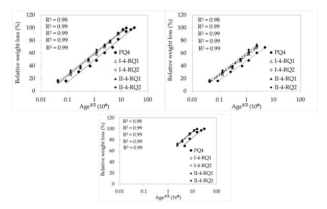
**Figure 8.** Relative weight loss vs. the square root of time for reference concretes. The slope of the curve represents the water release rate (WRR).
