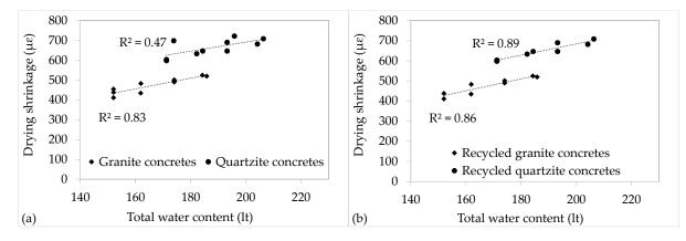
**Figure 7.** Relationship between drying shrinkage and total water content of reference and recycled concretes. (**a**) Reference and recycled concretes. (**b**) Only recycled concretes.
