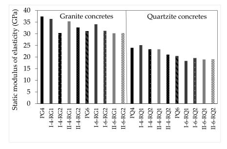
Figure 4. Static modulus of elasticity of concretes.
