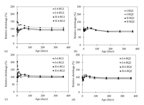
**Figure 6.** Drying shrinkage of recycled concretes relative to the reference concrete. (a) Granite recycled concretes, w/c = 0.40. (b) Quartzite recycled concretes, w/c = 0.40. (c) Granite recycled concretes, w/c = 0.55. (d) Quartzite recycled concretes, w/c = 0.55.
