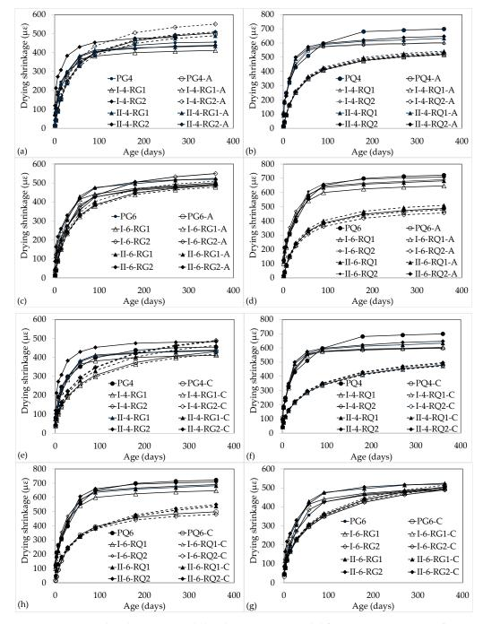
**Figure 9.** Estimated and experimental shrinkage. (a) ACI model for granite concretes, w/c = 0.40. (b) ACI model for quartzite concretes, w/c = 0.40. (c) ACI model for granite concretes, w/c = 0.55. (d) ACI model for quartzite concretes, w/c = 0.55. (e) CEB model for granite concretes, w/c = 0.40. (f) CEB model for quartzite concretes, w/c = 0.40. (g) CEB model for granite concretes, w/c = 0.55. (h) CEB model for quartzite concretes, w/c = 0.55.
