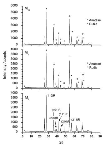
**Fig. 3** XRD pattern of TiO<sub>2</sub> nanopowders obtained through precipitation in microemulsion after calcination at 540 °C for 7 h in air flux:  $M_I$  (water/AOT/*n*-hexane, 30 °C),  $M_{II}$  (water/AOT/*n*-heptane, 30 °C), and  $M_{III}$  (water/AOT/cyclohexane, 30 °C). *R* rutile
