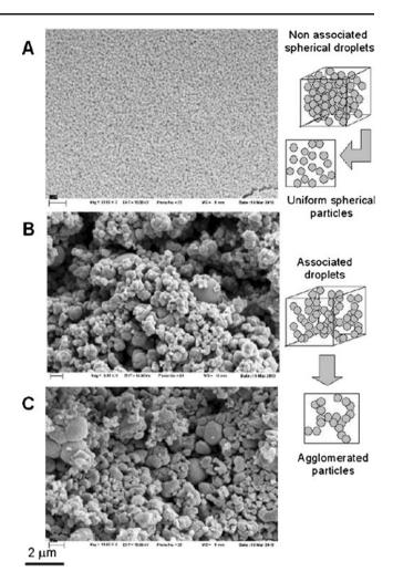
Fig. 1 FE-SEM microphotographs showing the surface morphology of  $TiO_2$  samples prepared by reverse microemulsions: **a** M<sub>I</sub>, **b** M<sub>II</sub>, and **c** M<sub>III</sub>
