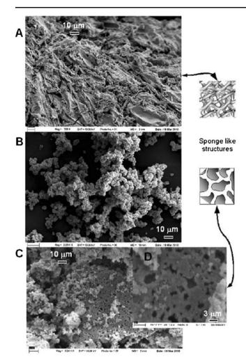
Fig. 2 FE-SEM microphotographs showing the surface morphology of TiO<sub>2</sub> samples prepared by reverse microemulsions: **a**  $M_{IV}$ , **b**  $M_{V_3}$  and **c**  $M_{VI}$
