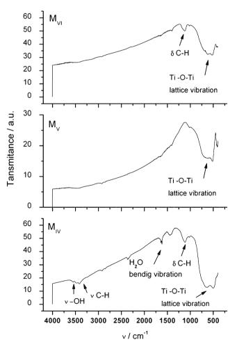
Fig. 6 FT-IR of TiO<sub>2</sub> samples.  $M_{IV}$  (water/AOT/*n*-hexane, 40 °C),  $M_V$  (water/AOT/*n*-heptane, 40 °C), and  $M_{VI}$  (water/AOT/cyclohexane, 40 °C)
