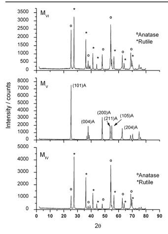
**Fig. 4** XRD pattern of TiO<sub>2</sub> nanopowders obtained through precipitation in microemulsion after calcination at 540 °C for 7 h in air flux:  $M_{IV}$  (water/AOT/*n*-hexane, 40 °C),  $M_V$  (water/AOT/*n*-heptane, 40 °C), and  $M_{VI}$  (water/AOT/cyclohexane, 40 °C). A anatase
