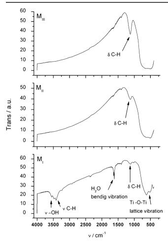
Fig. 5 FT-IR of TiO<sub>2</sub> samples.  $M_I$  (water/AOT/*n*-hexane, 30 °C),  $M_{II}$  (water/AOT/*n*-heptane, 30 °C), and  $M_{III}$  (water/AOT/cyclohexane, 30 °C)
