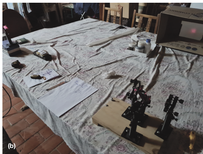
Fig. 3. (a) Close-up of the interferometer. (b) General arrangement: laser with pinhole, interferometer, and screen.
