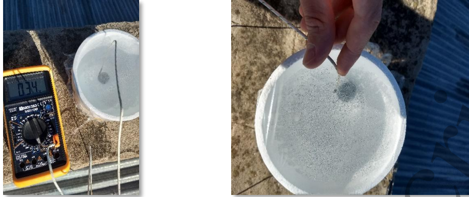
Figure 4: Glass samples in Styrofoam container covered with a plastic film. Thermocouple (K type) used to determine the temperature.
