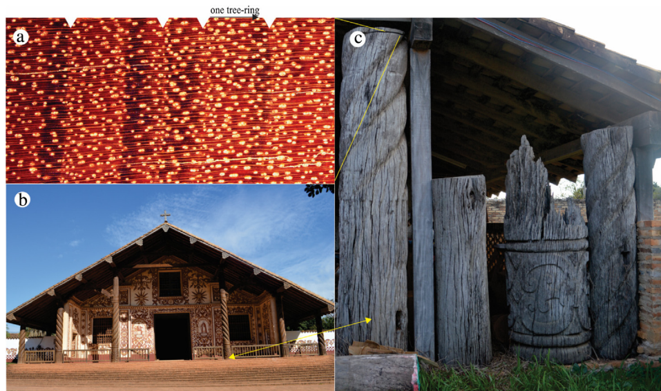
Fig. 3. Macroscopic structure of Schinopsis brasiliensis wood (a). Arrows indicate the boundary between consecutive rings marked by a thin line of marginal parenchyma (b). The restored Jesuit church of San Miguel Velasco, Velasco, Santa Cruz, Bolivia (c). Original S. brasiliensis columns salvaged from the church are stored in a local sawmill and were sampled for dendrochronology.
