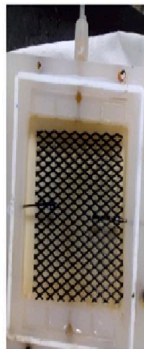
Scheme 1. Reactor scheme showing the electrolyte flow direction, electron current and ion fluxes. Right: Photo of a half compartment of the reactor.
