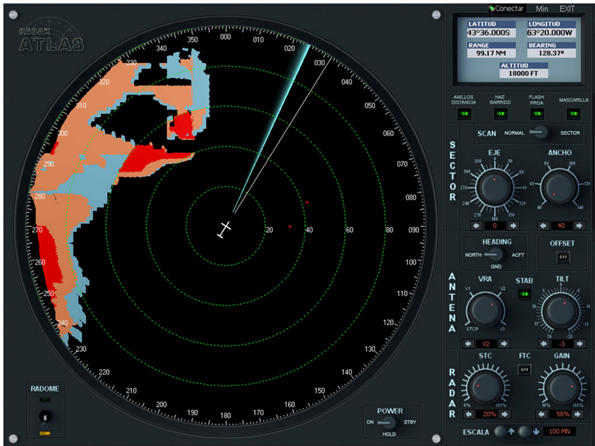
Figure 12 Colored echoes with a discrete color map. [Color figure can be viewed in the online issue, which is available at wileyonlinelibrary.com .]
