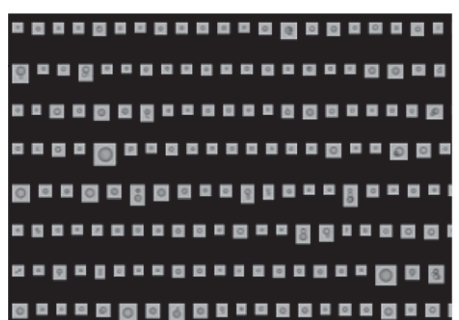
Fig. 10. Evaluation of the emulsion particle size by the Flow particle image analyzer (FPIA) in systems constituted by 10% w/w MCT oil and beetroot (3% w/w) or butternut pectin (4% w/w).
