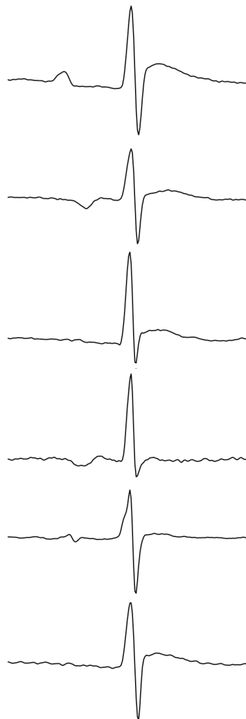
Fig. 2. Different ECG signals: From top to bottom, normal beat, inverted P-wave and symmetric QRS complex, without P-wave and asymmetric QRS complex, inverted P-wave and asymmetric QRS complex, biphasic P-wave, without P-wave and symmetric QRS complex.
