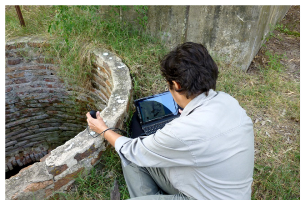
Figure 4 Dr. Mariel A López recording by USB microscopy the deterioration of the bricks of the edge of large water well located at the archaeological site SV2.
