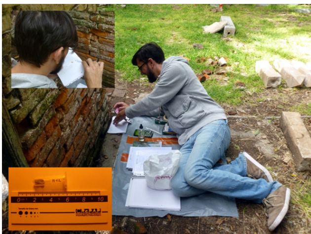
Figure 7 Magister Cristian López Rey sampling with scalpel, and occasionally using a consolidator (Paraloid), the different surface finishes previously mapped in survey cards on wall 4 of the archaeological site SV3. They were stored in small containers called eppendorf.
