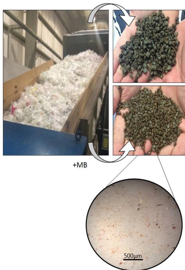
Fig. 1. Stages of recycling process of LLDPE/PP post-consumer (PCR) recycled blends and their impurities as observed by optical microscopy.
