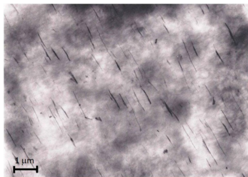
Figure 1. Transmission electron micrograph of polyethylene (PE) nanocomposite containing 1% by weight (wt%) sepiolite.
