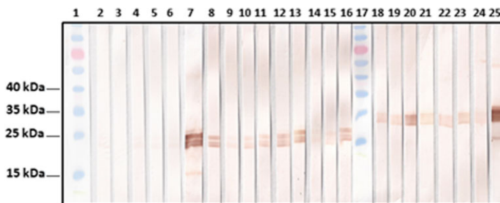
Fig. 6 Characterization of the p24 recombinant protein of BLV expressed in insect cells. The western blot analysis was carried out with a panel of representative cow sera. Lanes 1 and 17 : prestained molecular weight marker; lanes 2–6 : 1–5 sera samples from non-
