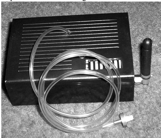
Fig. 6. Box containing one station and the battery. The box has a connector for the RF antenna and the tube to interface with the ETT cuff.
