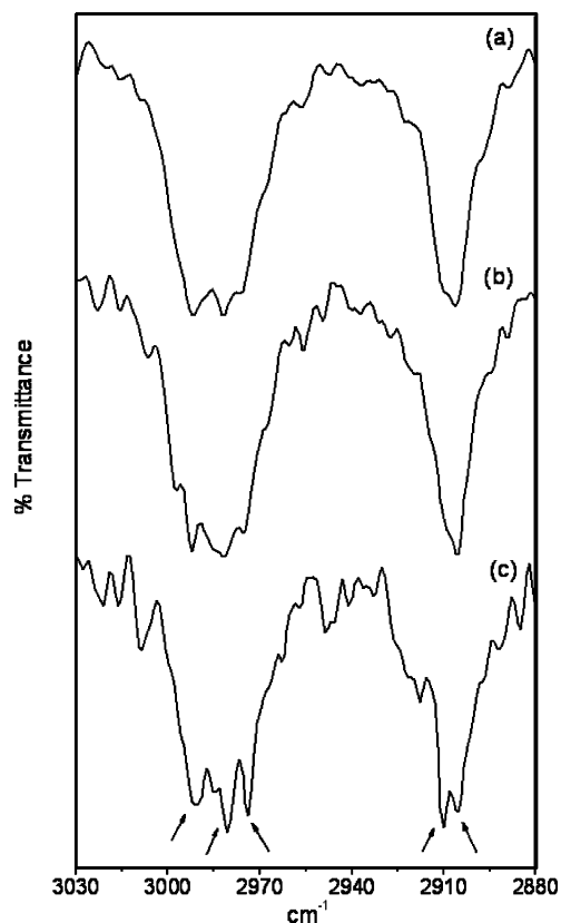
Figure 5. FTIR spectra of the region containing the CH 3 stretching modes at (a) room temperature, (b) -30 °C, and (c) -100 °C.
