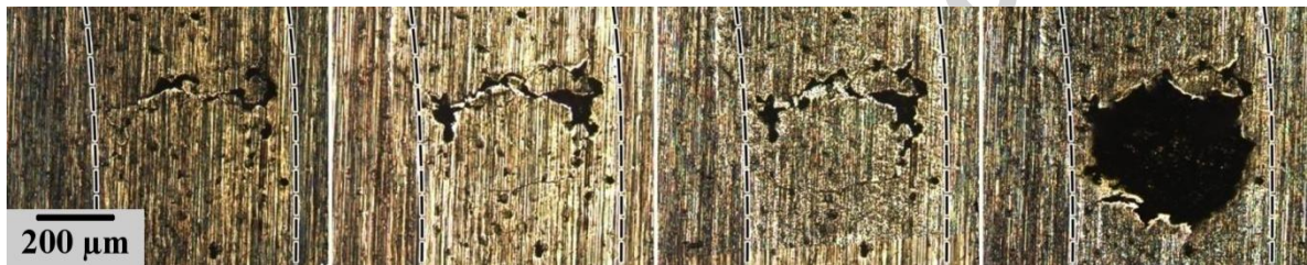
Figure 7. RCF failure evolution in ADI – AG
