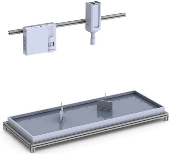
Fig. 1. Experimental setup to generate water wave turbulence. The tank of (200 \times 80) cm 2 is filled with water tainted with titanium dioxide to make it opaque and allow projection of a pattern on its surface. The two wavemakers driven by independent servomotors (not shown) excite random perturbations of the free surface. A high resolution projector projects a fringe pattern of known characteristics (not shown in the scheme), and a fast speed camera captures the pattern deformation. The profilometry technique then allows for reconstruction of the surface deformation with high temporal cadence and high spatial resolution [16, 17, 18].
