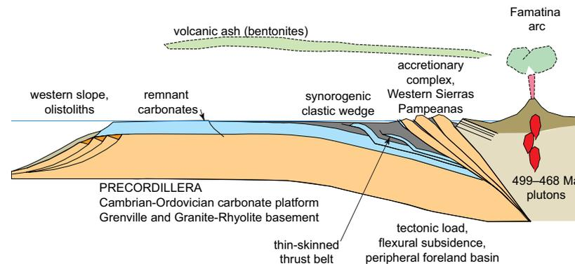
**Figure 11.** Diagrammatic cross section of tectonic model for the Middle–Late Ordovician foreland basin and clastic wedge in the context of accretion of the Precordillera to Gondwana and the Oclöyic orogeny.
