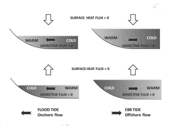
Figure 8. Schematic representation of the heat balance on an hourly scale. The shallower coastal area is warmed (cooled) more efficiently than the outer area when the surface heat flux is positive (negative). Consistent with flood (left) or ebb tide (right) the horizontal heat flow changes direction, accentuating or attenuating the effect of the atmospheric flow.
