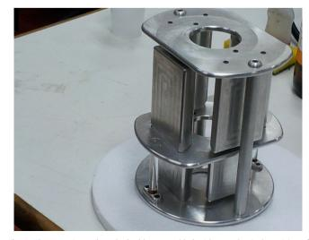
**Fig. 4.** Electrostatic quadrupole doublet, assembled with a mechanical precision of 0.01 mm.
