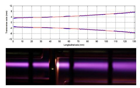
**Fig. 7.** Comparison between measured points of the beam profile (blue points) and the theoretical adjustment (red curve), in the upper part of the figure. Lower part: view of the same portion of the proton beam via the fluorescence induced in the residual gas propagating inside the quadrupole channel. (For interpretation of the references to color in this figure legend, the reader is referred to the web version of this article.)
