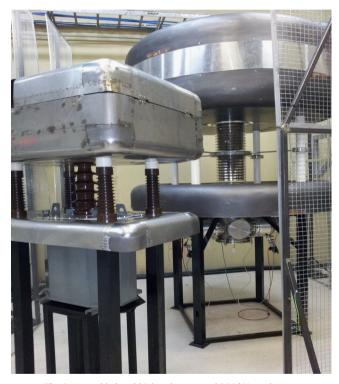
Fig. 2. Assembled and high-voltage tested 200 kV accelerator.
