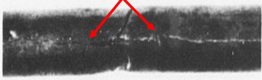
Figure 2(a) Field and laboratory fracture shapes of pre-stressing wires with crack-like laminations (US Bureau of Reclamation, 1994). (a) First fracture shape described as cup and cone failure with a metal tongue; (b) Second fracture shape unidentified by USBR [12].
